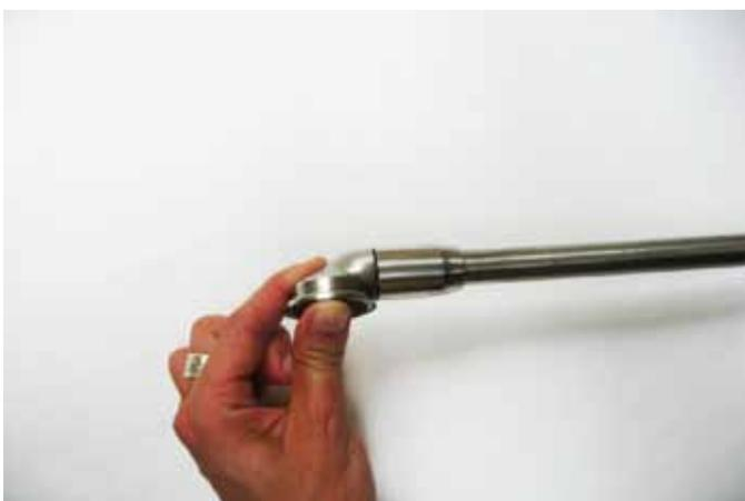
The head is correctly positioned when it reaches the notch and you hear a click.
