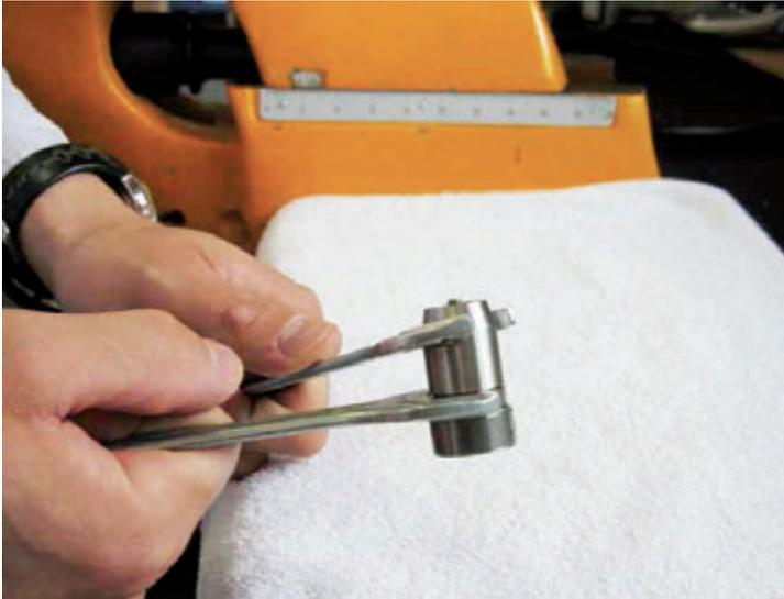
Unscrew the nut carry-bearing from the ball-holder ring with tool n°4.
