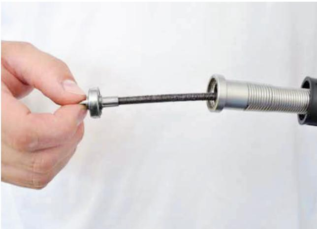
Remove piece D by the tips of the drive shaft connected to the engine
