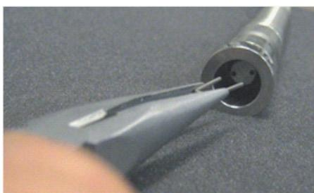
*Shear pin replacement using pliers*
