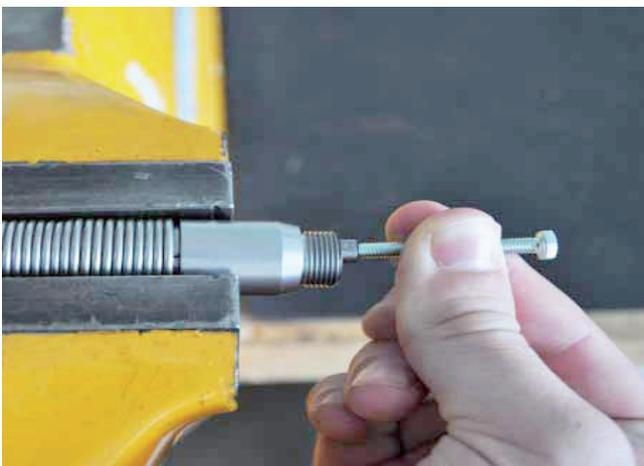
Screw tool n°1 on the drive shaft
