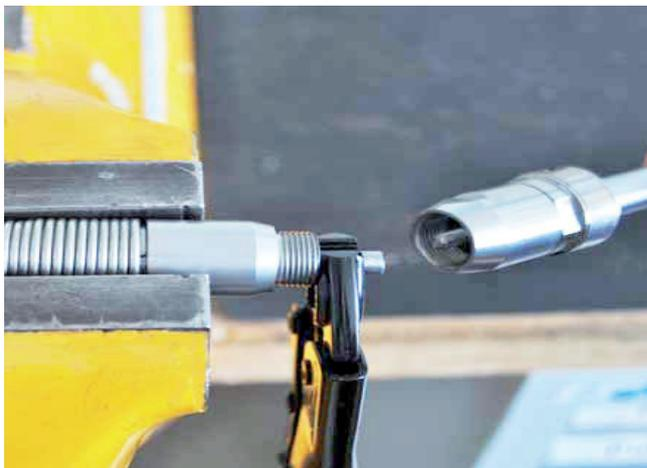
Screw the new piece B on the inner cable with tool n°3 (*slightly* tighten).
