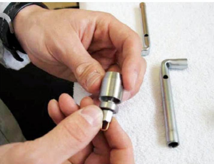
Remove the 2 holes driving screw.
