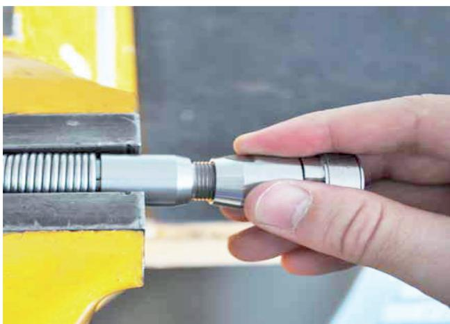
Remove tool n°3 & screw piece B on piece C.
