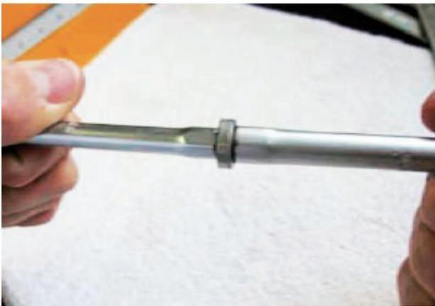
Unscrew the nut from the screw to change the bearing and screw back everything with tools n°3 & 3 bis.
